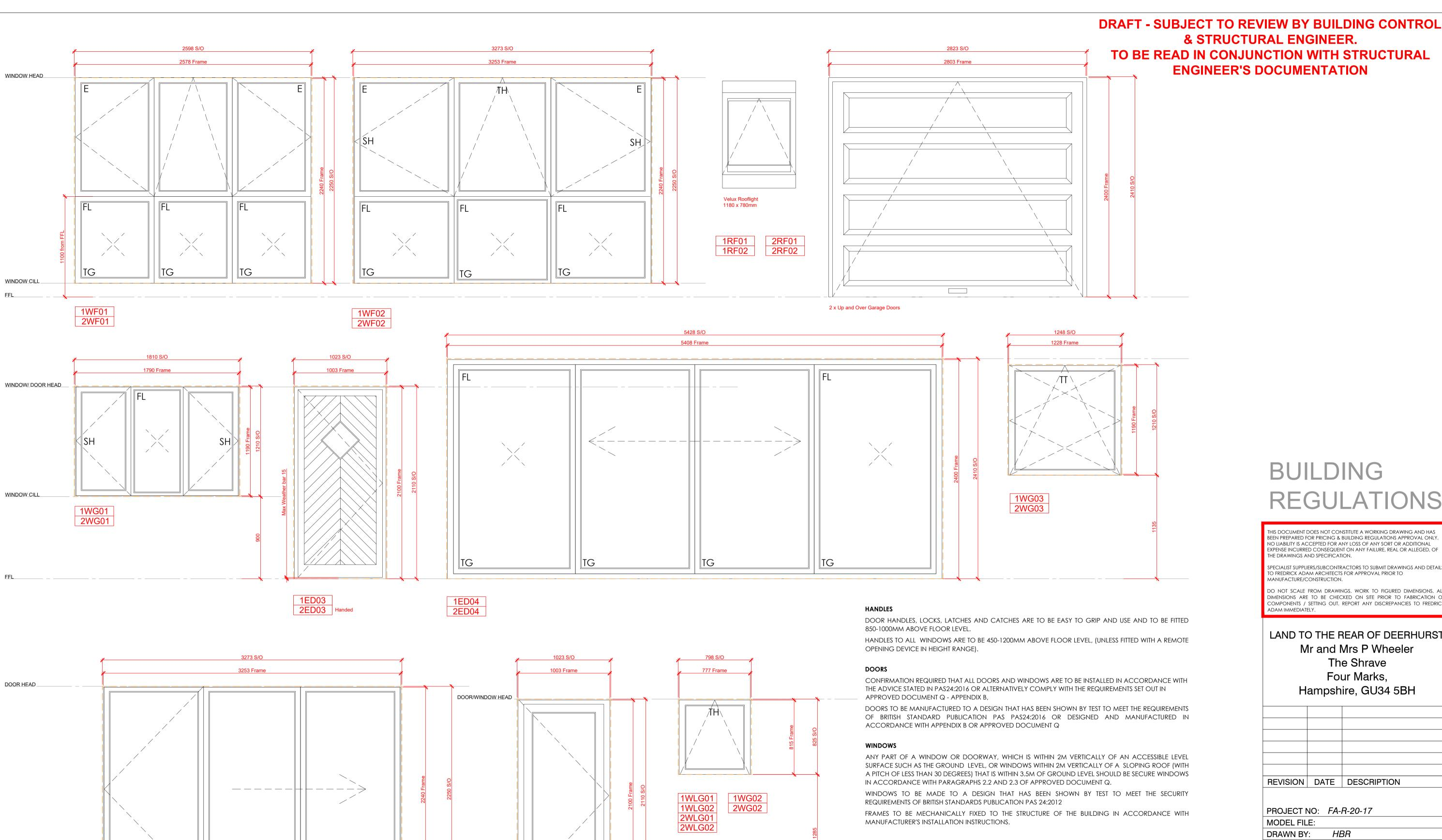
STRUCTURAL TOLERANCES TO BE CONFIRMED WITH MANUFACTURER PRIOR TO ORDER. ALL DIMENSIONS TO BE CONFIRMED ON SITE PRIOR TO ORDER - ALTERNATIVELY SACRIFICIAL FRAMES TO BE CONSTRUCTED AND BUILT IN ACCORDANCE WITH GIVEN DIMENSIONS. IT IS THE RESPONSIBILITY OF THE CONTRACTOR AND WINDOW SURVEYOR TO CONFIRM ALL OPENINGS AND SIZES PRIOR TO ORDER. WINDOW SCHEDULE FOR PRICING ONLY.
