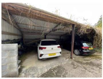
42' 0" x 22' 0" (12.80m x 6.71m) of steel frame construction with 3 separate bays providing Garage and vehicular parking space, concrete base, box profile cladding to side and to roof.
