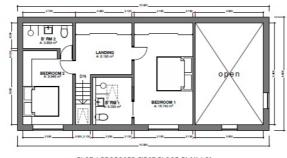
PLOT 1 PROPOSED FIRST FLOOR PLAN 1:50
