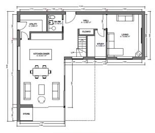
PLOT 2 PROPOSED GROUND FLOOR PLAN 1:50
