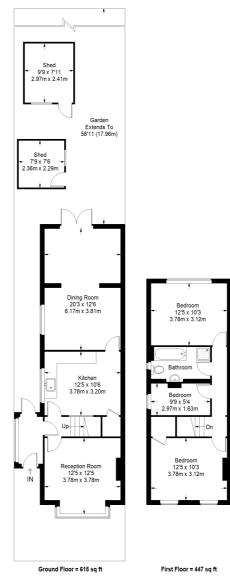
Approximate Gross Internal Area GROUND FLOOR = 615 sq ft / 57.13 sq m FIRST FLOOR = 447 sq ft / 41.53 sq m SHED = 136 sq ft / 12.63 sq m Total = 1198 sq ft / 111.29 sq m
