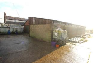
**Stable Block** (45' x 20') (Building No. 5 on site plan) A concrete brick and block built mono pitch building with box profile tin roof sheeting over a concrete floor used as stabling for 4 horse stables in fabricated removable partitions.
