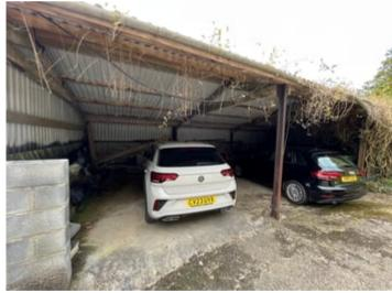
42' 0" x 22' 0" (12.80m x 6.71m) of steel frame construction with 3 separate bays providing Garage and vehicular parking space, concrete base, box profile cladding to side and to roof.
