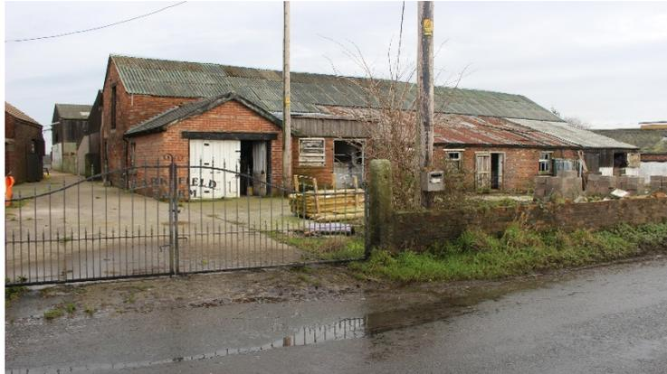
**Ex Parlour** (75' x 20') A mono pitch leanto building constructed from concrete block and red brick to part and a corrugated tin sheet roof. Internally the building has a concreted floor, concrete block stables.
