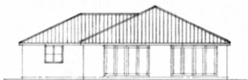
PROPOSED REAR ELEVATION UPVC BI-FOLD DOORS TO CLIENT'S SPECIFICATION
