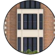
Stonework surrounding bay windows, and coining details.
