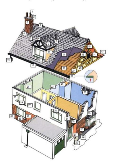
Ridge ventilation 5 Ridge board Slates/tiles 8 Valley guttering 9 Dormer projection Dormer flashing 10 Dormer cheeks 11 12 Sarking Roof felt 13 Trusses 14 15 Collar 16 Insulation 17 Parapet gutter Eaves guttering 18 Rainwater downpipe 19 20 Verge boards / skews 21 Soffit boards 22 Partition wall Lath / plaster 23 24 Chimney breast 25 Window pointing Window sills 26 Rendering 27
