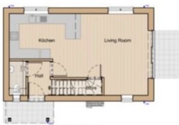
GROUND FLOOR PLAN GIA FLOOR AREA - 39 Sq m - 424 Sq ft TOTAL DWELLING GIA FLOOR AREA - 78 Sq m - 848 Sq ft
