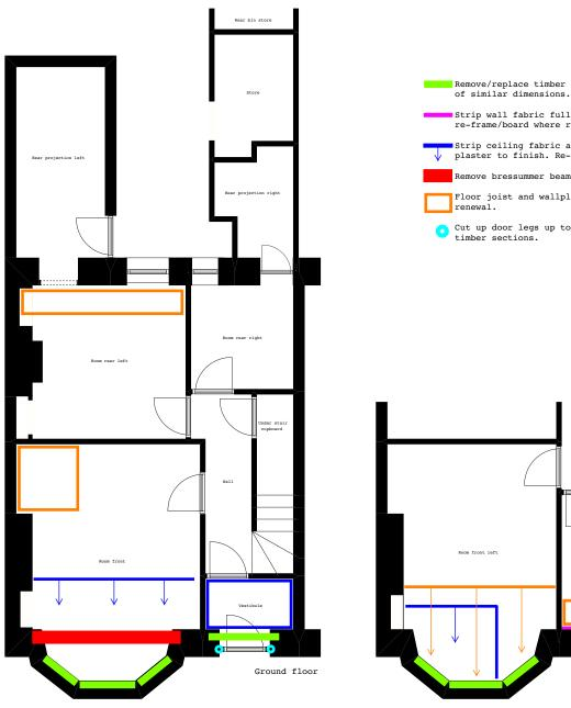
Remove/replace timber safe lintels with concrete lintels Strip wall fabric full height, fix cavity drain membrane, re-frame/board where required and plaster to finish. Strip ceiling fabric and cornice. Fix new plasterboard and plaster to finish. Re-run cornice to match existing. Remove bressummer beam and replace with steel beams. Floor joist and wallplate repairs and floorboard removal/
