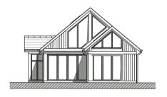
Proposed Roof Structure, Fibre Cement Slate, Clay Vented Ridge, Upvc Fascia and Soffits Upvc Rain Water Goods. PPC Aluminium Rough Sawn Treated Softwood Stained Cladding, Staff, Blue Engineering Brick Plinths.
