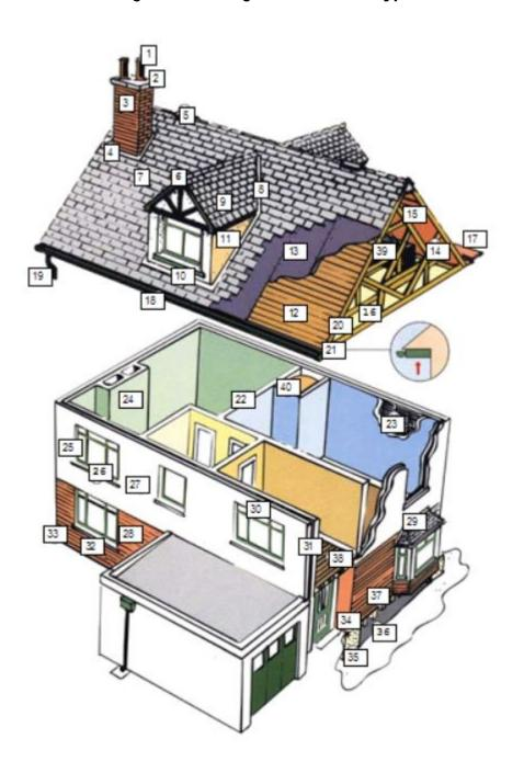
Ridge ventilation 5 Ridge board Slates/tiles 8 Valley guttering 9 Dormer projection Dormer flashing 10 Dormer cheeks 11 12 Sarking Roof felt 13 Trusses 14 15 Collar 16 Insulation 17 Parapet gutter Eaves guttering 18 Rainwater downpipe 19 20 Verge boards / skews 21 Soffit boards 22 Partition wall Lath / plaster 23 24 Chimney breast 25 Window pointing Window sills 26
